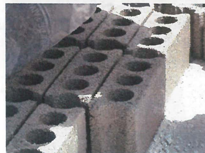
A smooth and regular finish on the top and sides shows good compaction throughout the block
